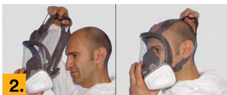
2. Pull the face respirator down over the head placing the nose and chin in the nose cup/chin area. Then press the facepiece firmly and evenly against the face. Pull head harness to back of head.
