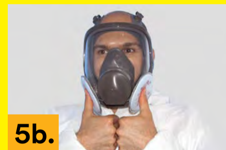
5b. With Particulate Filters – Disc Style: Place your thumbs onto the centre portion of the filters to restrict the air flow. Inhale gently. The facepiece should collapse slightly.
