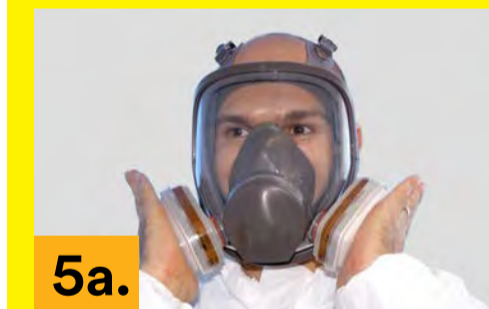
5a. With cartridges: Place the palms of your hands over the cartridge to restrict air flow. Inhale gently. The facepiece should collapse slightly.
