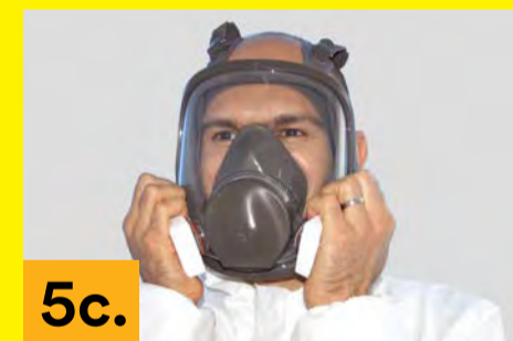
5c. With Solid-top Particulate Filters: Squeeze filter covers together using the palms of your hands and fingers to restrict airflow. Inhale gently. The facepiece should collapse slightly.
